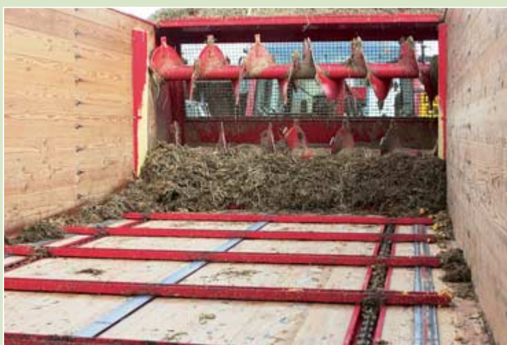
The Foster forage box holds about 6t of feed. According to the Myatts, the box is a much quicker and more fuel efficient way of feeding the cows when compared with a diet feeder.
