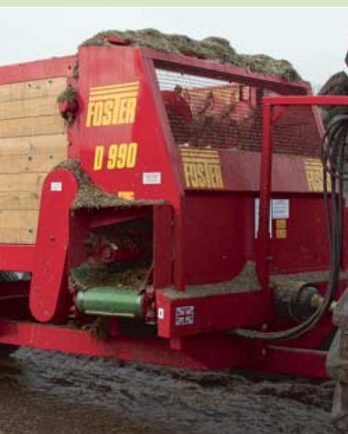
The Foster forage box holds about 6t of feed. According to the Myatts, the box is a much quicker and more fuel efficient way of feeding the cows when compared with a diet feeder.
