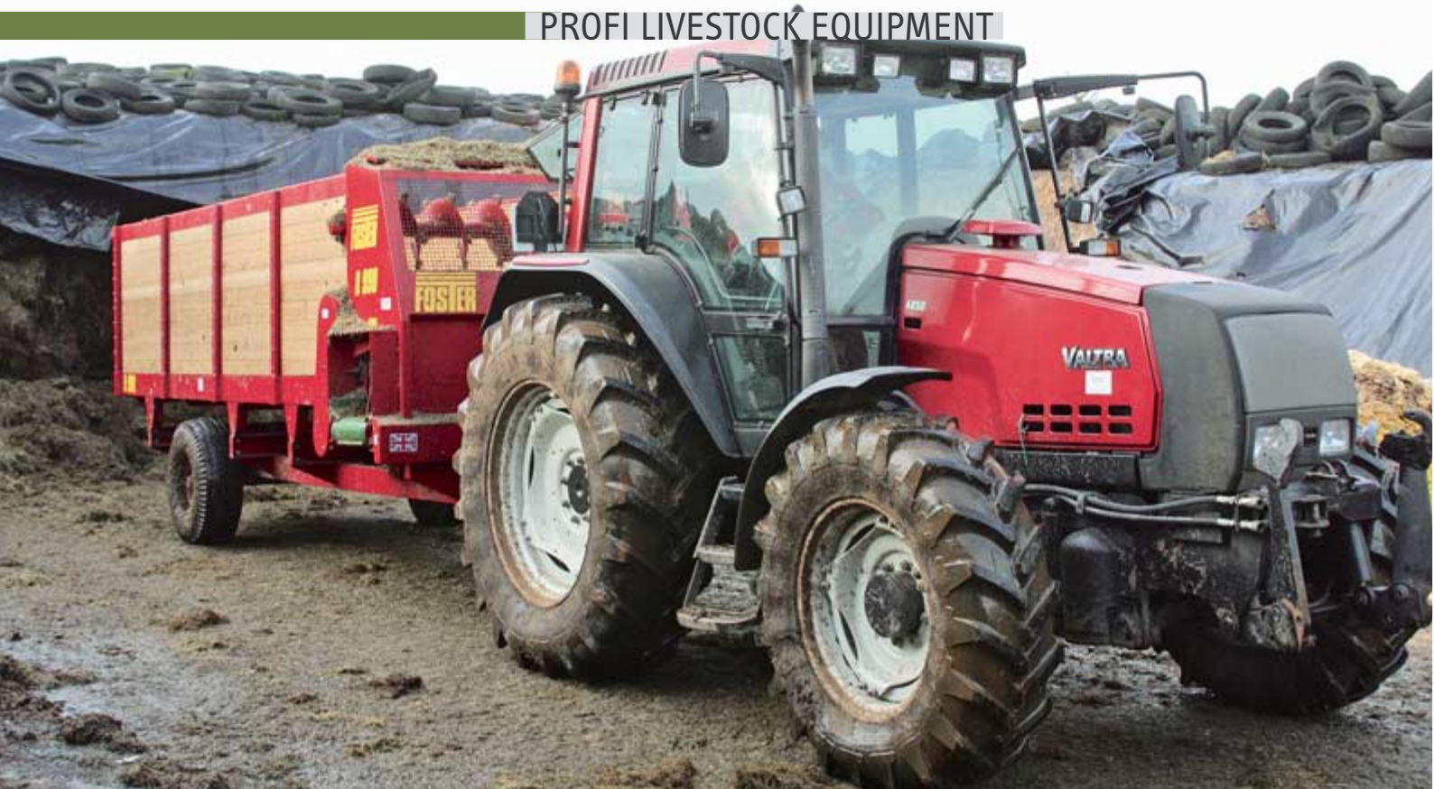
The Foster forage box offers a more traditional approach to dairy cow feeding. Here, box muscle is provided by a 93kW/125hp Valtra 6850.
