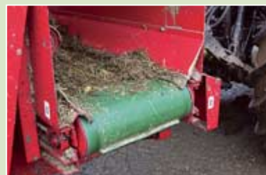
Mr Myatt has noticed a significant drop in fuel consumption since moving from a diet feeder to a simple forage box. Above: Belt conveyor is capable of discharging to either side.
